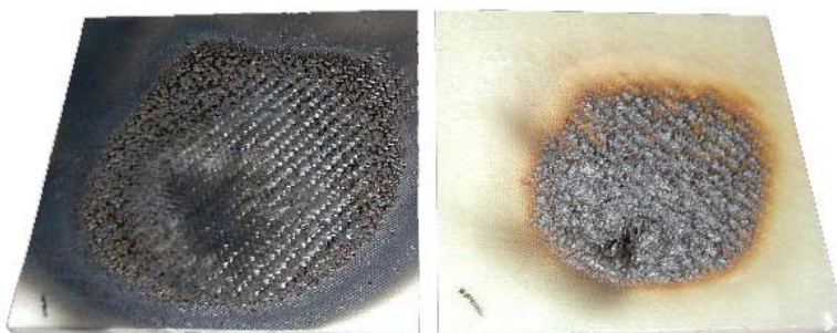
E glass laminates after test burning: Brominated epoxy / Intumescent epoxy
